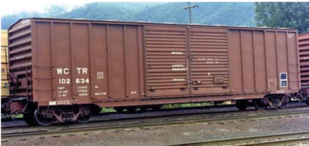
White City Terminal 100-ton boxcars, frequently found in Siskiyou Line trains, were notorious for "slip joints." —Bruce Petty
