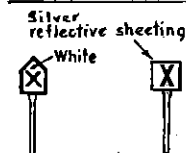
HIGHWAY GRADE CROSSING WHISTLE SIGN
