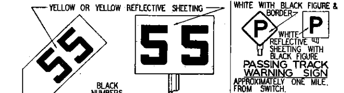
PERMANENT ADVANCE WARNING SIGN LOCATED APPROXIMATELY ONE MILE FROM POINT SPEED RESTRICTION EFFECTIVE. RULE 10 (h) PERMANENT SPEED RESTRICTION SIGN LOCATED AT BEGINNING OF RESTRICTION.
