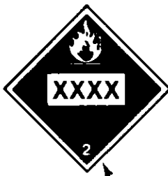
NUMBER 2 FLAMMABLE GAS
