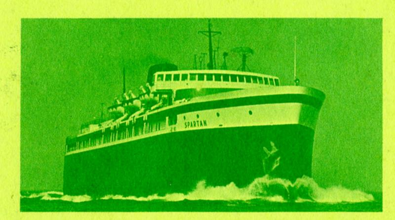
The Spartan, Badger and City of Midland have a speed of 18 miles an hour and can carry 500 passengers, 26 railroad cars and 25 to 50 automobiles. The ships are air conditioned and equipped with the latest safety devices including radar, radio direction finders, ship-to-shore telephones and many water-tight bulkheads. The bows of the ships are reinforced to serve as ice breakers during the winter months.
