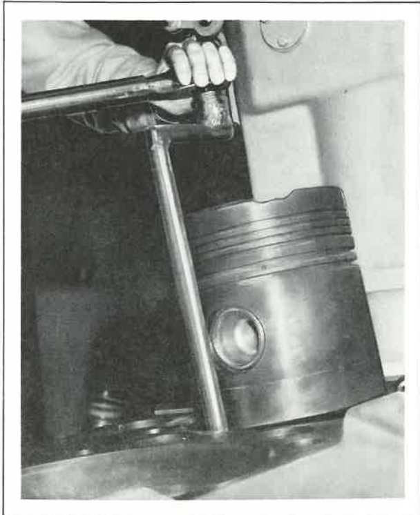
FIG. IX-72. LOOSENING PISTON PIN BOLTS.
