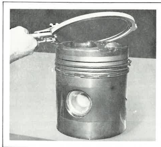
FIG. IX-74. APPLYING RINGS WITH RING EXPANDER TOOL.
