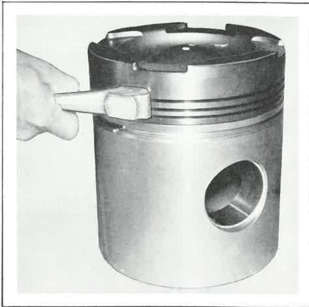
FIG. IX-69. CLEANING PISTON RING GROOVE WITH SCRAPER, PART 147X1098.
