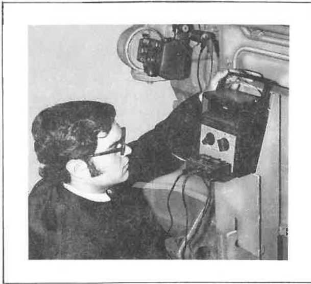
FIG. XI-18. MEASURING ENGINE SPEED AT TACHOMETER DRIVE FITTING ON GOVERNOR DRIVE GEAR BOX.
