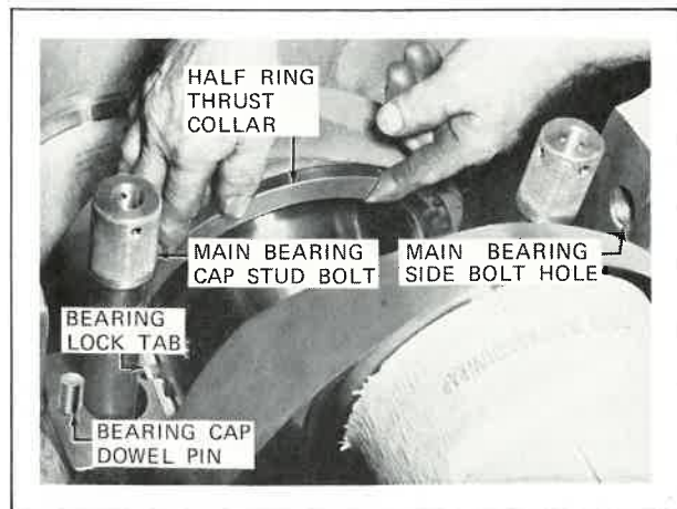
FIG. IX-87. INSTALLING THRUST COLLARS.
