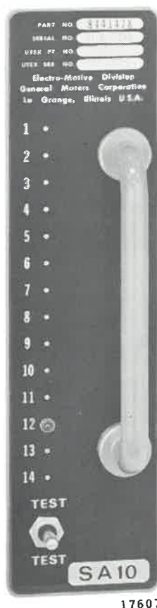
Fig. 5-19 - Sanding Circuit Module
