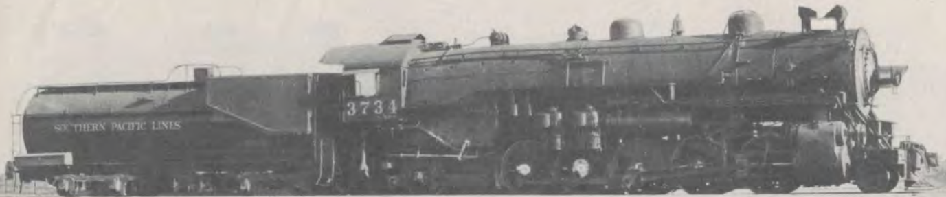
This is a 2-10-2 Type Locomotive. It is Used to Pull Freight Trains
